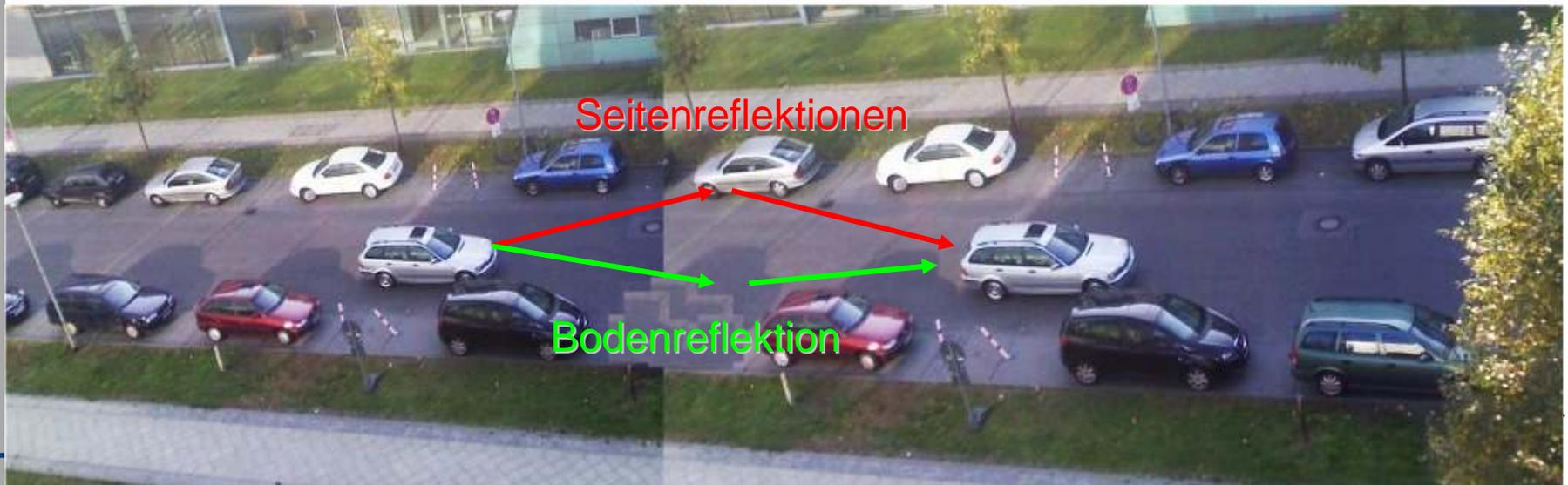
$$h = \sqrt{\frac{L\lambda}{4} + \frac{\lambda^2}{16}} \sim \sqrt{\frac{L\lambda}{4}} \quad L \sim \frac{4h^2}{\lambda} \quad \lambda = \frac{c}{f}$$
